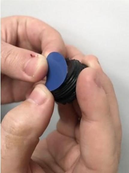
To remove air bubbles trapped between the sensing patch and sensor surface, gently roll your thumb over the applied patch from one side of the sensor to the other.
